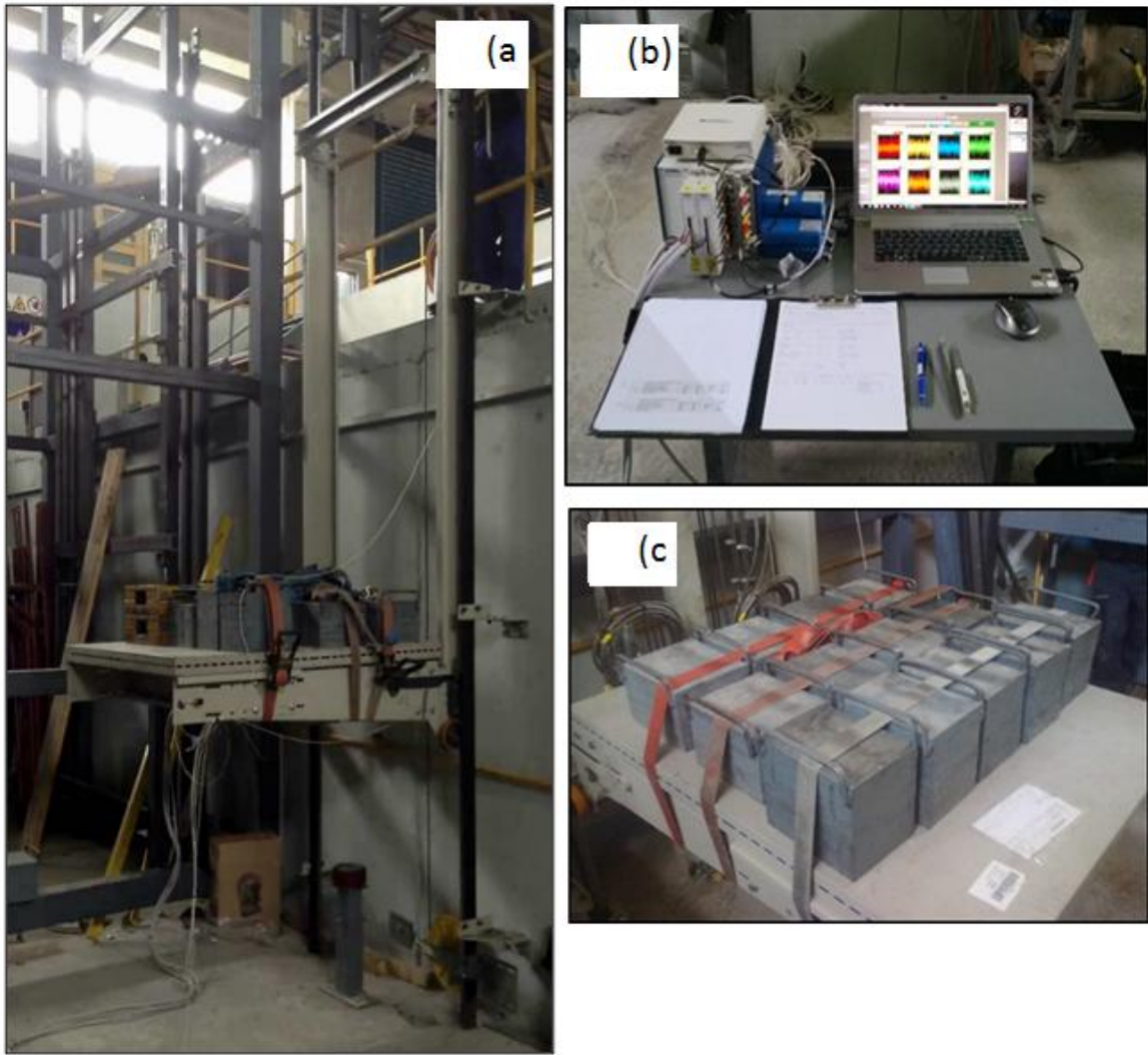
Fig. 32 - (a) Experimental device, (b) Data acquisition system, and (c) Elevator platform with load
