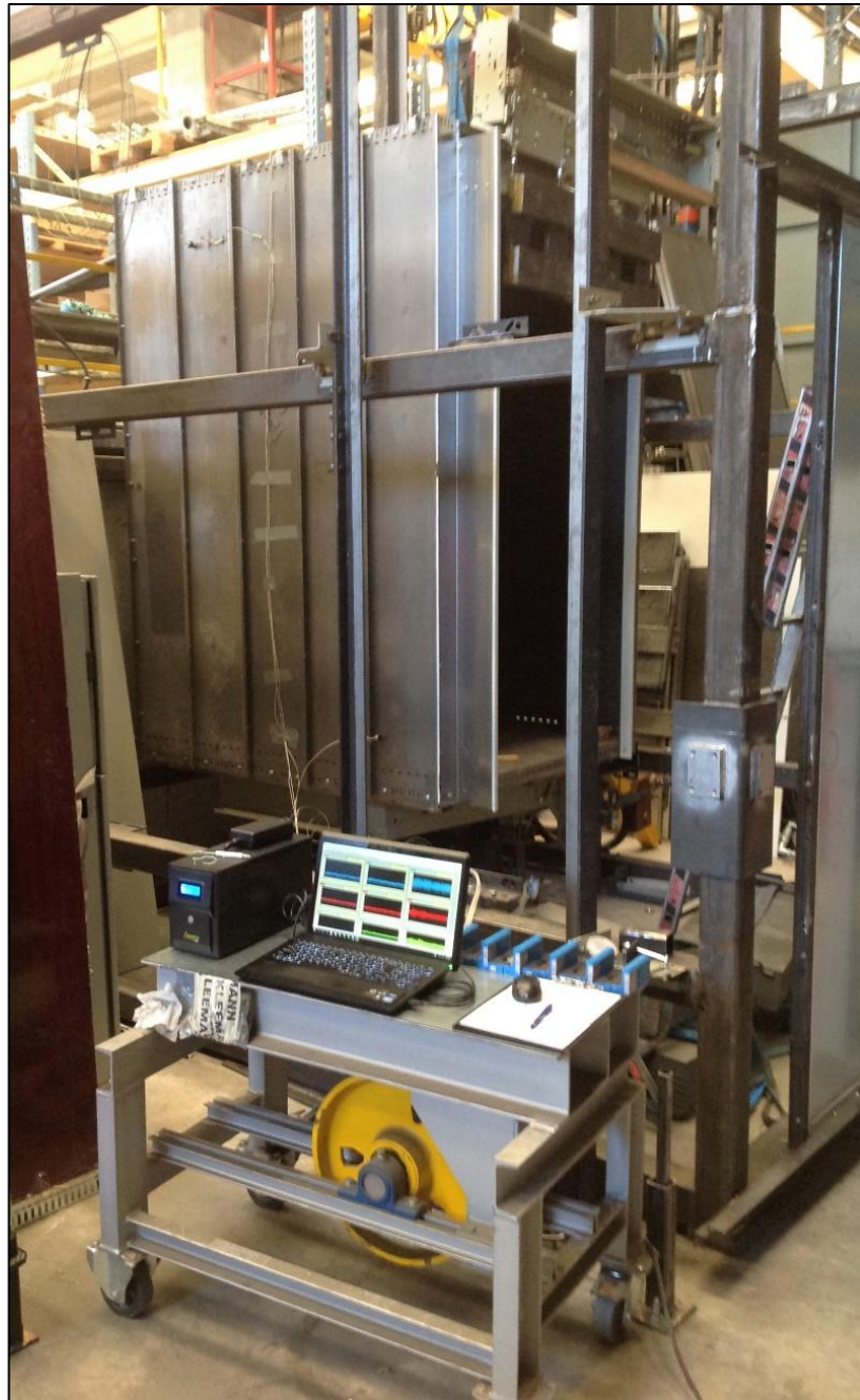
Fig. 47 - Experimental set up of the complete elevator system
