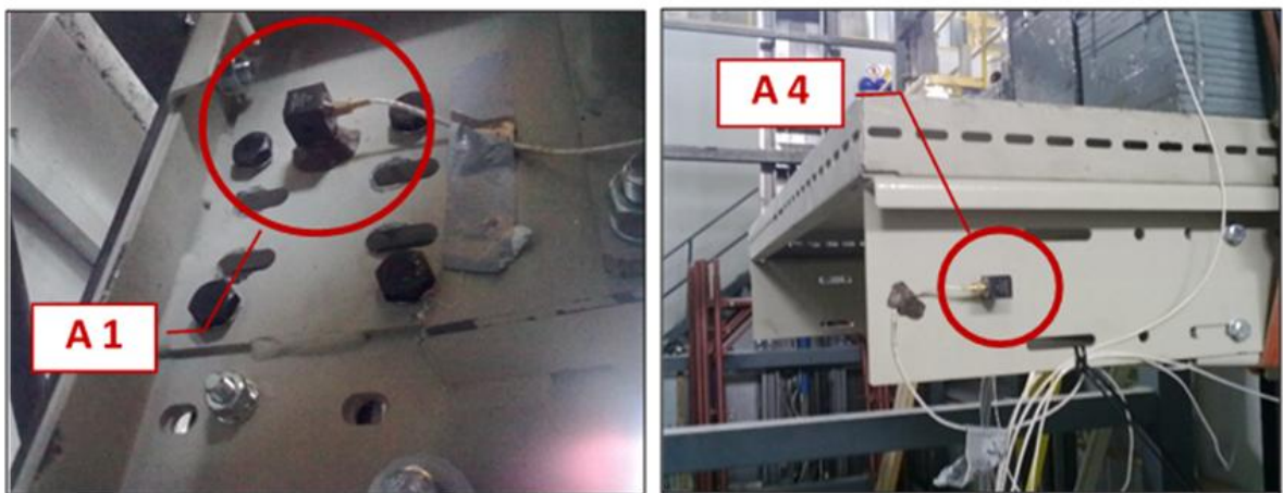
Fig. 33 - Acceleration measurement locations at a connection point (A1) and at a reference point (A4)
