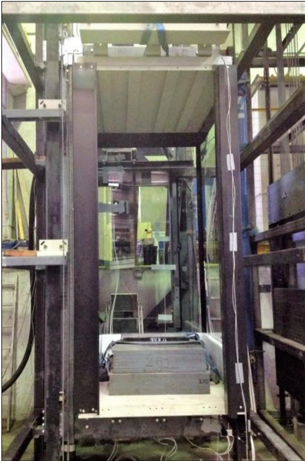
Fig. 59 - Full Glass Frameless Car Experimental Verification Set Up
