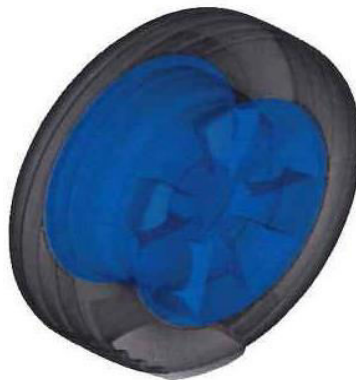
Figure 4.4: Wheel with highlighted MRF/SM region enclosing the spokes
