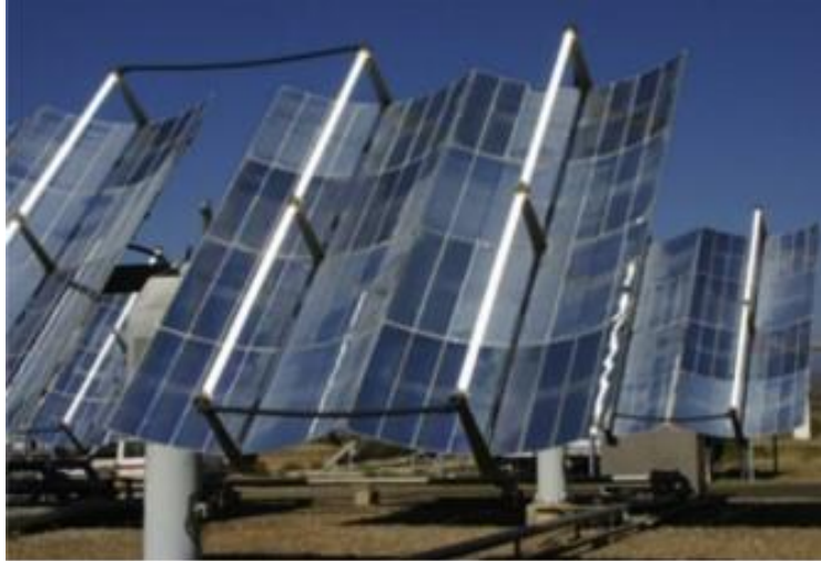
Εικόνα 5.3 SOLARIS: Κυλινδρικός συλλέκτης. Πηγή: Danilo Spasiano, Raffaele Marotta, Sixto Malato, Pilar Fernandez-Ibanez, Ilaria Di Somma (2015). “Solar photocatalysis: Materials, reactors, some commercial, and pre-industrialized applications. A comprehensive approach”. Applied Catalysis B: Environmental , 170-171, pp. 90-123 https://doi.org/10.1016/j.apcatb.2014.12.050
