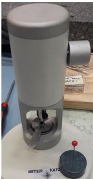
Figure 18. Left: Clamping device for DSC pans. Right: DSC sample tray
