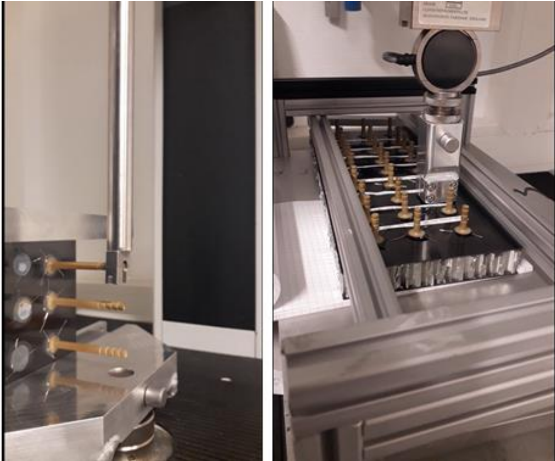
Figure 39. Left: Shear mode testing. Right: Tension mode testing
