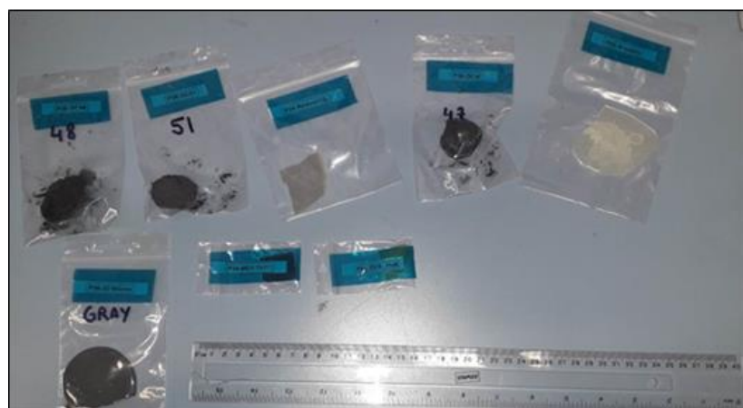
Figure 4. Cured adhesives for material characterization
