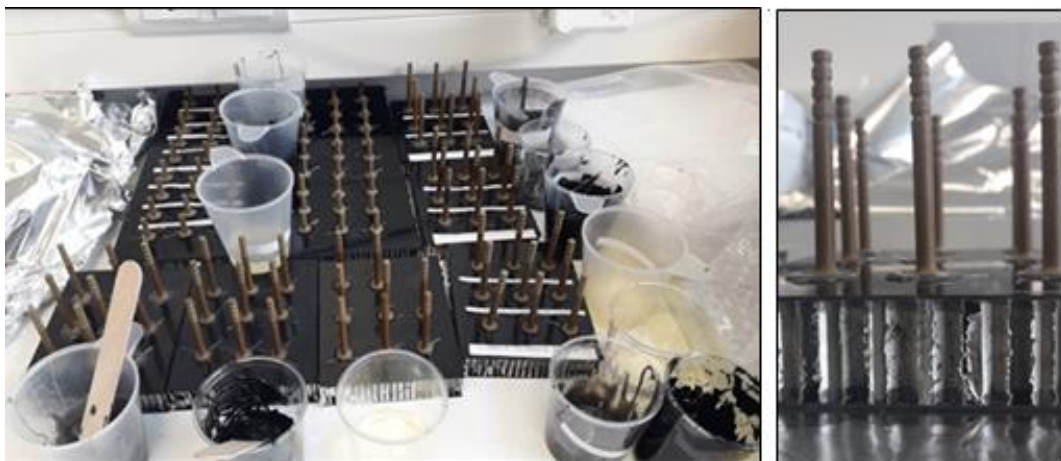
Figure 33. Standoffs and extra adhesive curing in room temperature
