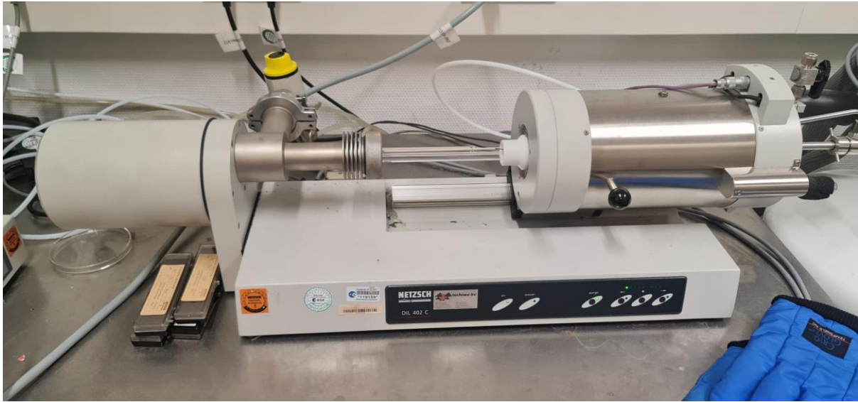
Figure 21. DIL 402C instrument
