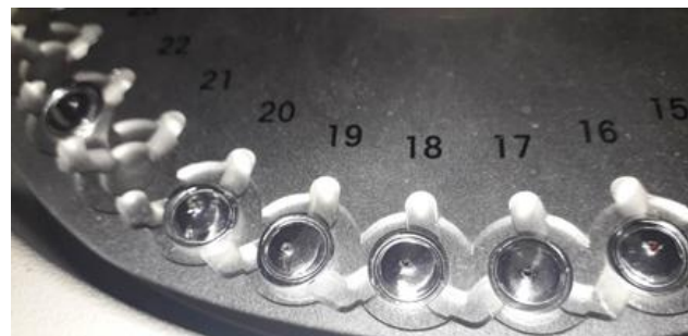
Figure 18. Left: Clamping device for DSC pans. Right: DSC sample tray
