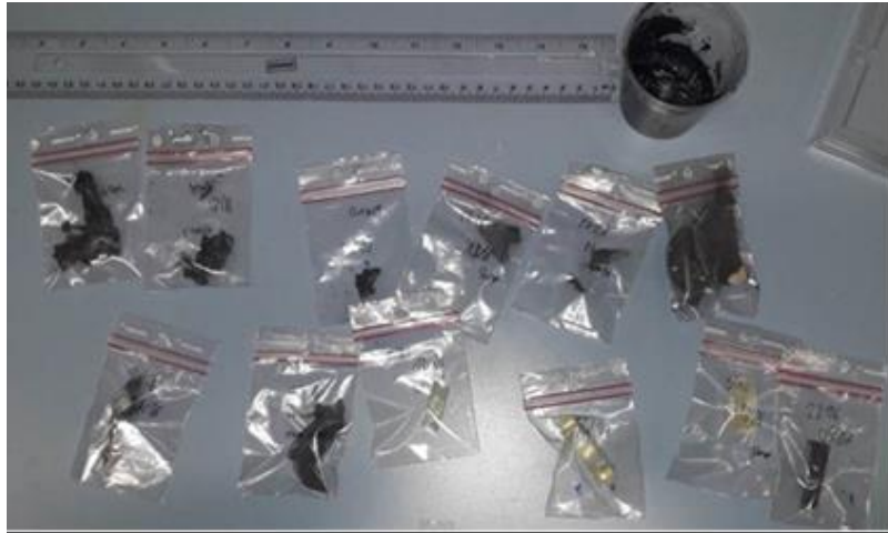
Figure 5. Standoff bonding cured adhesives for DSC test
