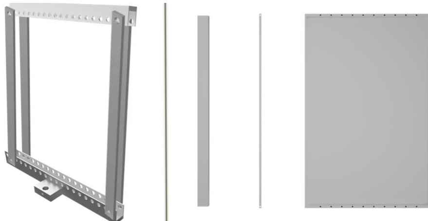
Figure 36. Initial jig concepts. Left: Shear jig. Right: Tension jig.
