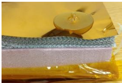
Figure 2. An MLI standoff holding the MLI blanket to the substrate (5)
