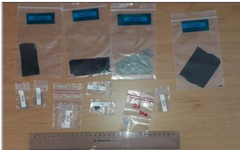
Figure 3. Examples of cured film adhesives for material characterization
