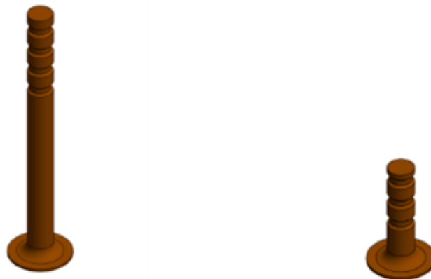
Figure 15. Left: Standoff used for shear testing. Right: Standoff used for tension testing
