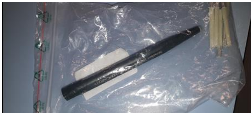
Figure 30. Fiber-glass pen used for sanding
