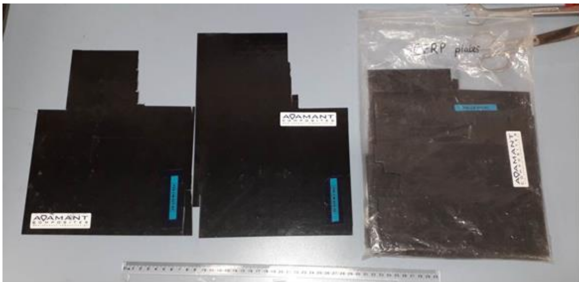
Figure 12. CFRP plates used for material characterization
