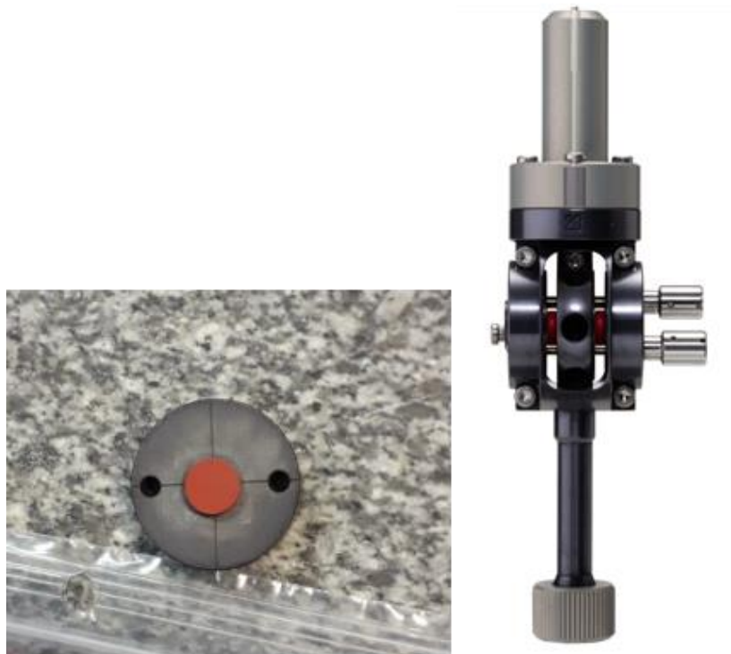
Figure 28. Left: DMA sample preparation in shear. Right: DMA Shear mode set up
