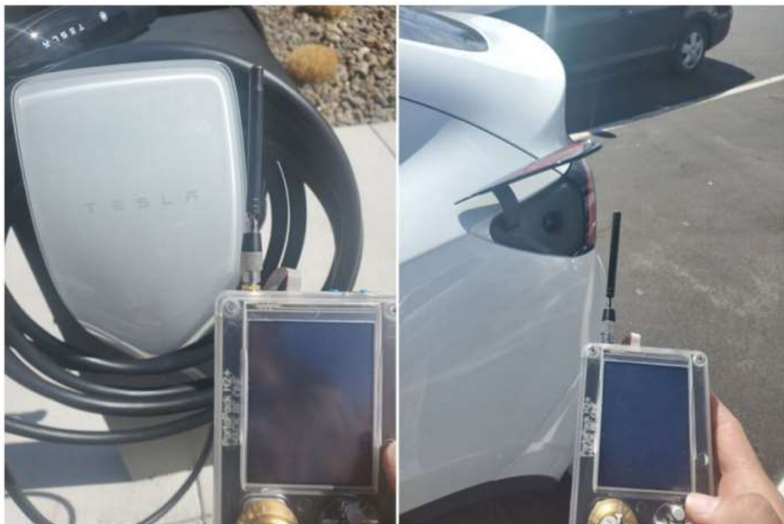
Tesla Charging Port Opened with HackRF and Portapack | Credit: @IfNotPike
