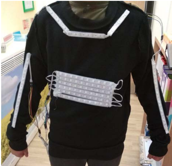
Figure 15. The wearable e-textile. LED strips and LED matrix screen.
