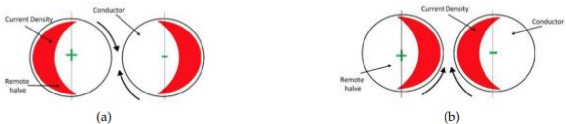
Figure 12: Representation of current density if the current flows (a) in the same direction, (b) in the opposite direction.
