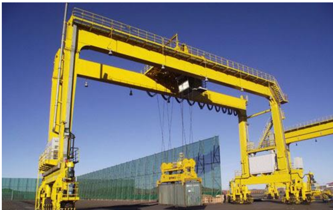
Figure 4. Rubber Tired Gantry Cranes (RTG)
