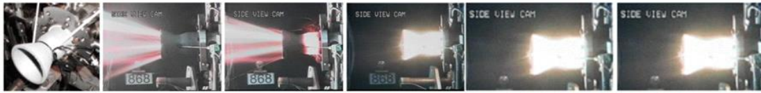
Ultramet carbon fiber-reinforced zirconium carbide combustion chamber during 4350°F (2400°C) hot-fire testing at NASA Glenn
