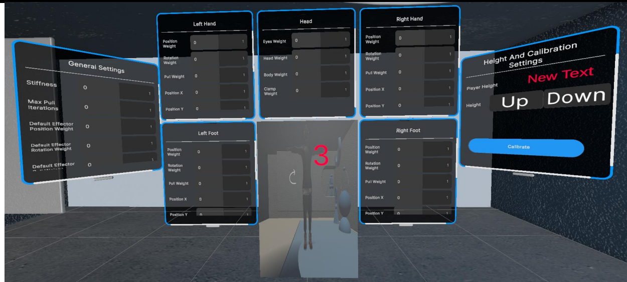
Figure 28: The VR IK Editor for modifying the effector properties on runtime and perform calibration method.
