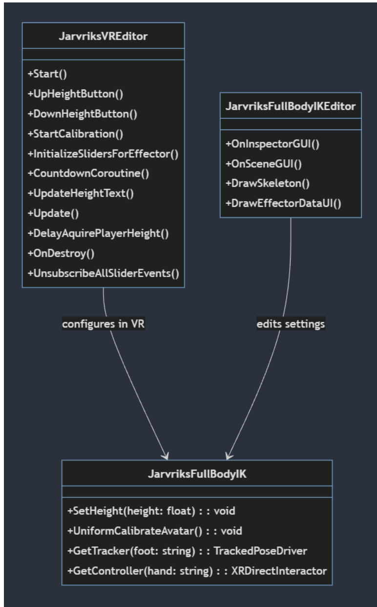
Figure 26: The JarvriksVREditor and JarvriksFullBodyIKEditor class diagram with their relation to the JarvriksFullBodyIK class
