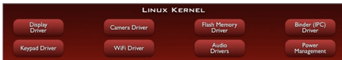
Figure 1.2:20-Linux kernel in Android Operating System
