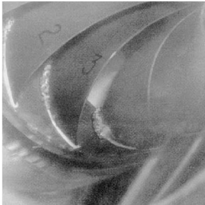
Εικόνα 16-Τύπος σπηλαιώσης leading edge cavitation. ΠΗΓΗ: "Investigation of a Francis turbine during speed variation: Inception of cavitation"
