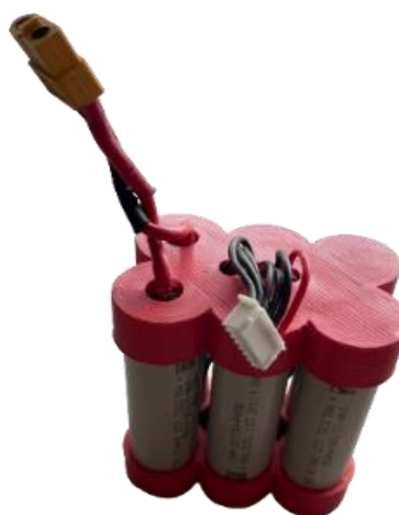
Figure 8 Battery pack connecting 6 single cell batteries
