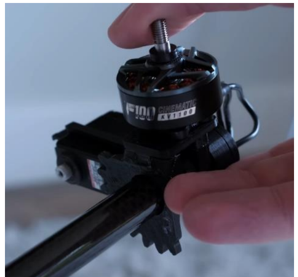
Figure 26 Assembling the motor in the servo mechanism
